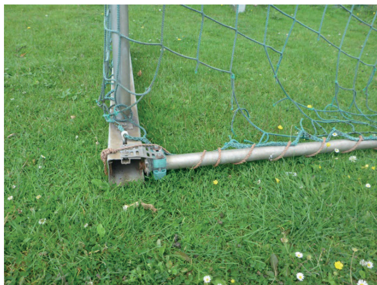
Risk of injury from open rear ground bar with sharp edges.
